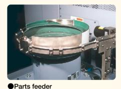
This is a bucket type stocker suited to small workpieces that do not take up much space. The part feeder can be directly linked to a conveyor.
