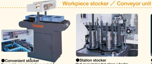
Reasonably priced and allows control of workpiece transport in bucket units.
