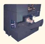
Chip conveyor (Spiral type) Enables semi-automated chip disposal in the minimum space.
