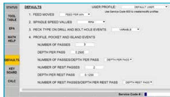
Defaults teach the ProtoTRAK RX your machining style
